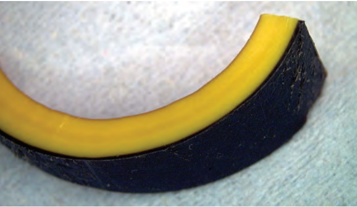
Historical yellow polyethylene (PE) gas service pipe with black outer layer of lead and lead sulfide. Due to the black discoloration, the live gas pipe was misidentified as a water pipe and was cut open causing a gas leak. Lead pigments are no longer used in modern polyethylene pipes.
